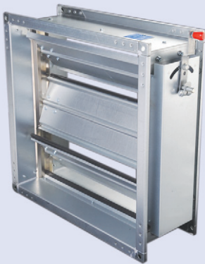
C3: construction with profiled dampers and silicone seal, which meets the requirements of resistance to high temperatures of 280 °C/ 1 h
